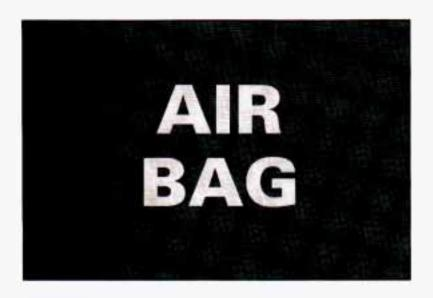
You will see this light flash for a few seconds when you turn your ignition to RUN or START. Then the light should go out. This means the system is ready.
